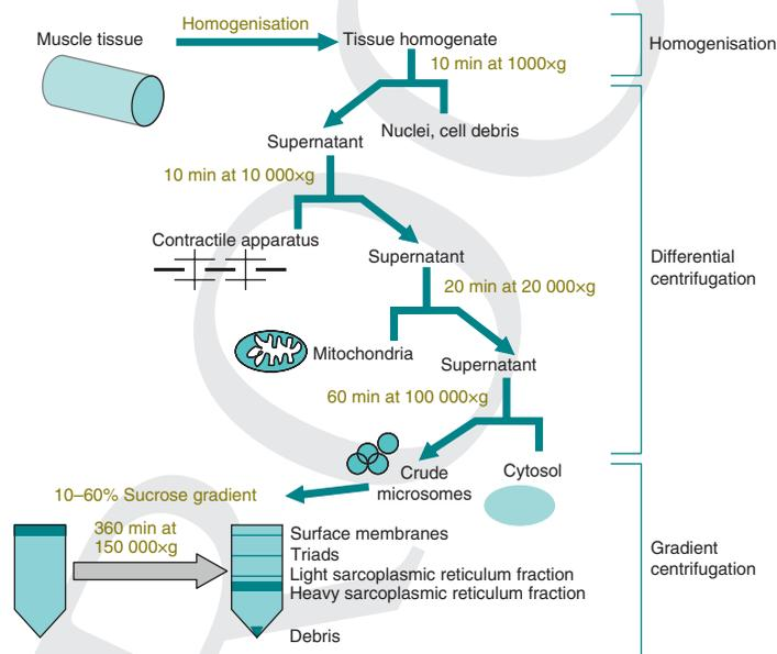
Figure 12.5 Scheme of the fractionation of skeletal muscle homogenate into various subcellular fractions. Shown is a diagrammatic presentation of the subcellular membrane system from skeletal muscle fibres (a) and a flow chart of the fractionation protocol of these membranes from tissue homogenates using differential centrifugation and density gradient methodology (b).
