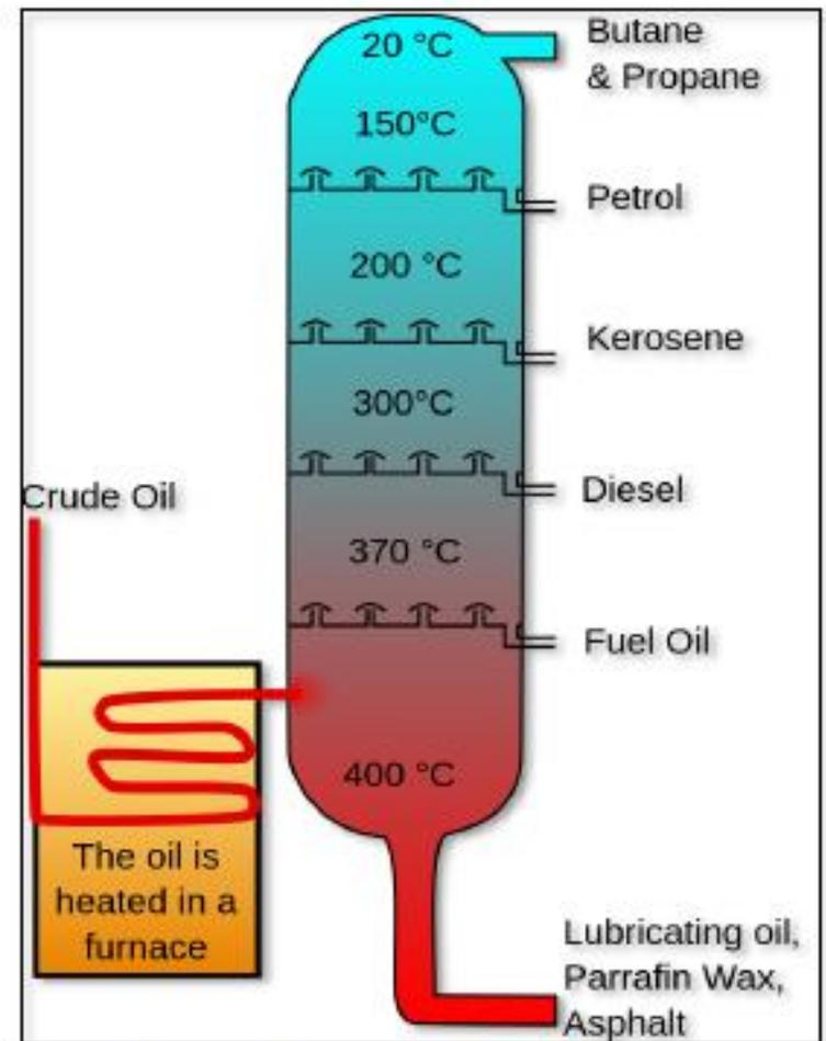
Distillation of crude oil in a distillation tower.
