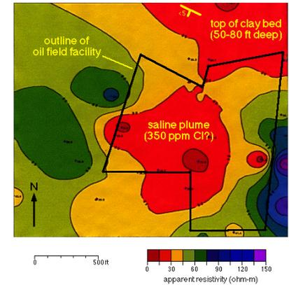
Contour map of apparent resistivity in vicinity of oil field facility corresponding to a Schlumberger electrode spacing (AB/2) of 100 ft. Contour map is representative of hydrology and geology at a depth of 50-80 feet. Interpretations are supported by well data and computer models of resistivity data.
