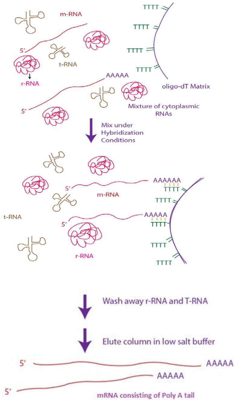
Figure 4-3.2.1. Isolation of mRNA using oligo-dT column chromatography.
