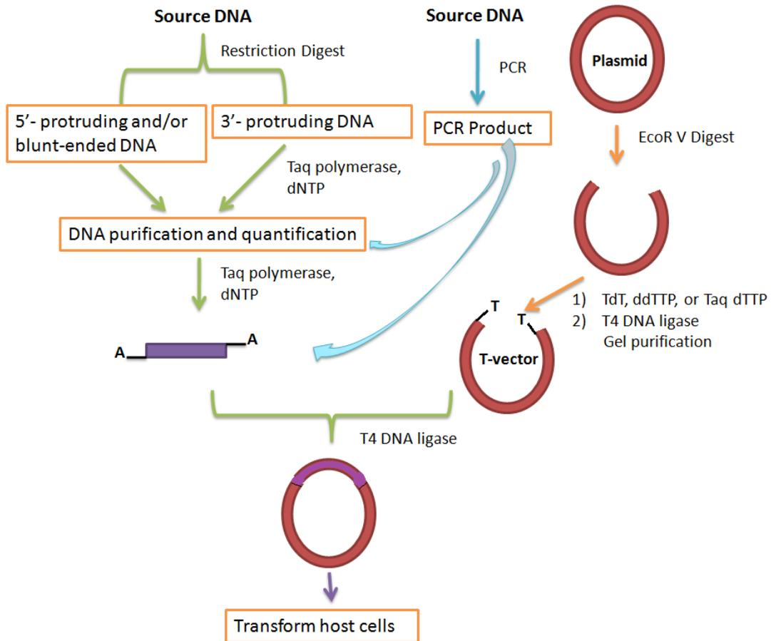
Figure 4-6.2.1(a) Schematic representation of the cloning procedures using the universal T-vectors
