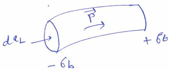
Let change in electric polarization produces the flow of bound charge ( $J_p$ )
