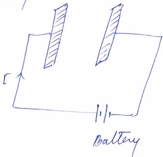
The current flowing in the ~~capacitor~~ conducting wire is equal to the rate of change of charge on the plates
