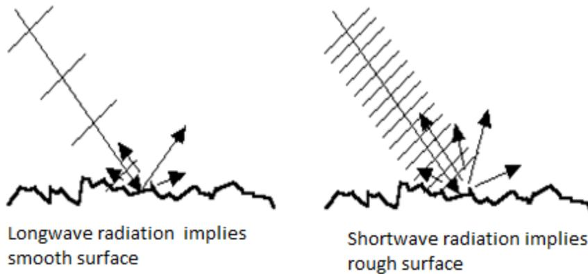
Fig 4. Comparison of smooth and rough surfaces
