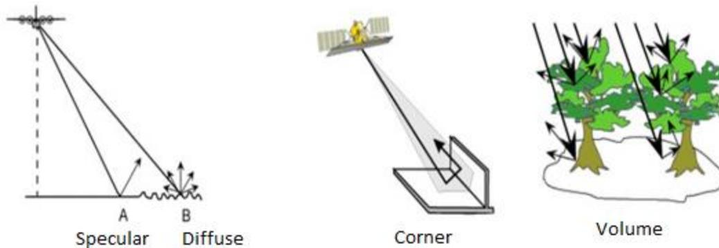
Fig. 6 Illustration of the various scattering scenarios
