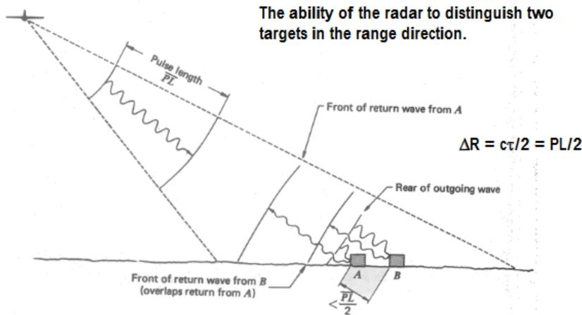
Fig 1. Range resolution is dependent on pulse length
