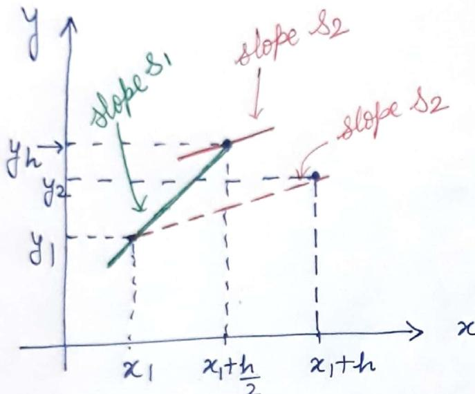
We start a line with slope  $s_1 = f(x_1, y_1)$  from point  $(x_1, y_1)$ .
