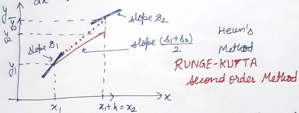
Here a straight line is drawn from point  $(x_1, y_1)$  with a slope  $s_1 = f(x_1, y_1)$ . Let it cut the vertical line through  $x_1 + h$  at  $(x_1 + h, \bar{y}_2)$ .
