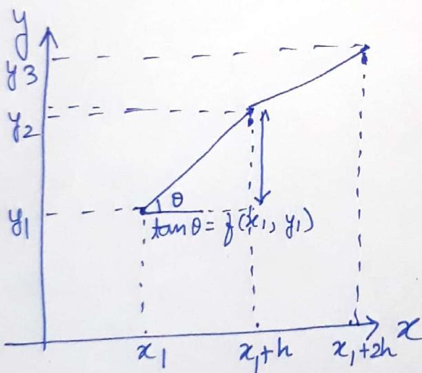
The next point  $y_2$  on the solution curve may be extrapolated by taking a small step ( $h$ ) in a direction given by the above slope eq<sup>M</sup> (3).
