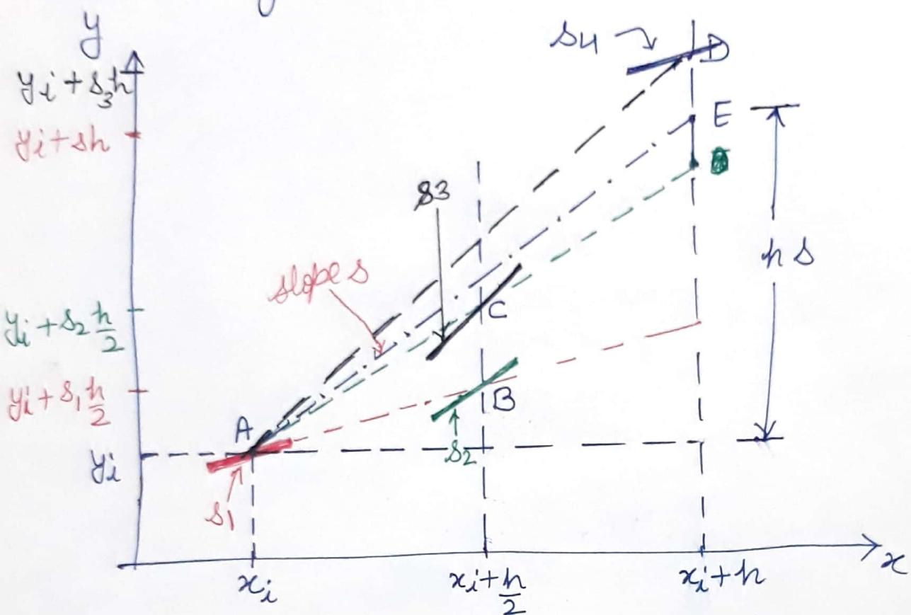
We draw a straight line from point  $A(x_i, y_i)$ , with slope  $s_1 = f(x_i, y_i)$ . Let this straight line cut the vertical line erected at  $(x_i + \frac{h}{2})$  at  $B$ .
