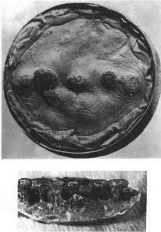
Figure 12.8 Model of mantled gneiss dome structure produced in a centrifuge experiment. Domes of stitching wax in putty overburden are developed along the boundary of a deep-seated, less dense, source layer. Diameter of model 94 mm. The lower photograph shows a sideways view with the putty overburden removed. The domes are outlined in ink. This experiment simulates the effect of gravity in causing the diapiric uprise of less dense material into a denser overburden. (From Ramberg, H. (1962) Bulletin of the Geological Institute of the University of Uppsala , 42, figures 27 and 28.)
