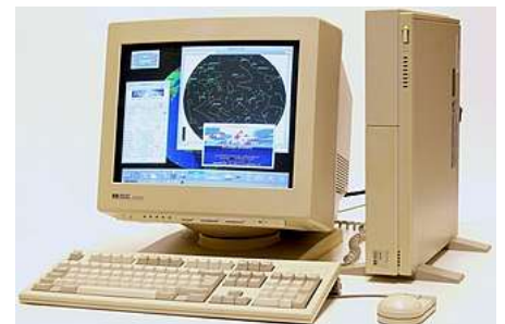
HP 9000 model 425 workstation running HP-UX 9 and Visual User Environment (VUE)
