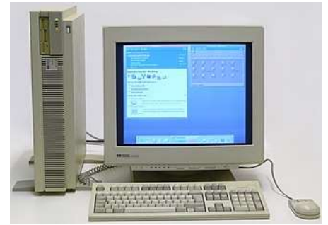
HP 9000 model 735 running HP-UX and the Common Desktop Environment (CDE)
