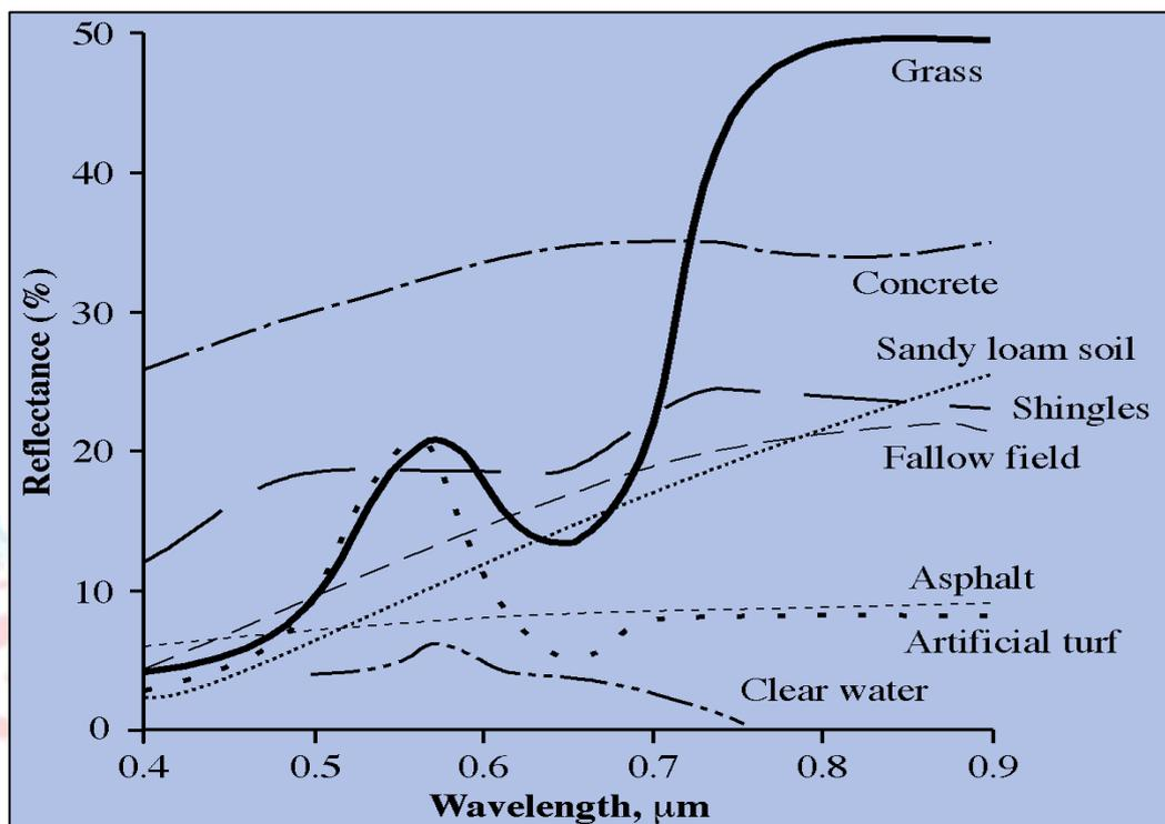
**Fig. 5** Typical Spectral reflectance curves for various Earth's surface features.
