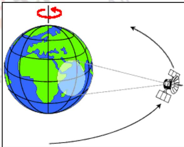
**Fig. 10** Geostationary orbit.
