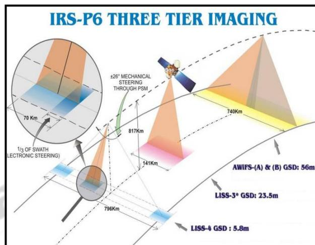
**Fig. 1** Indian remote sensing platform and sensor.
