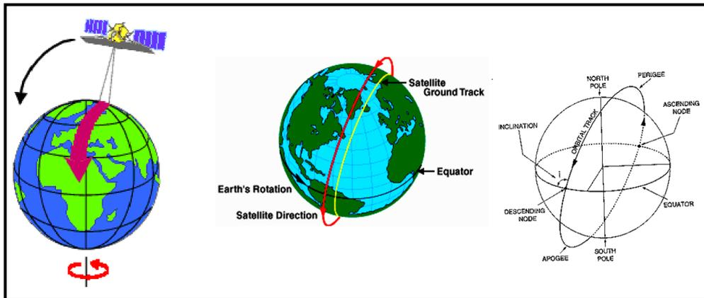
**Fig. 8** Sun-synchronous orbit.
