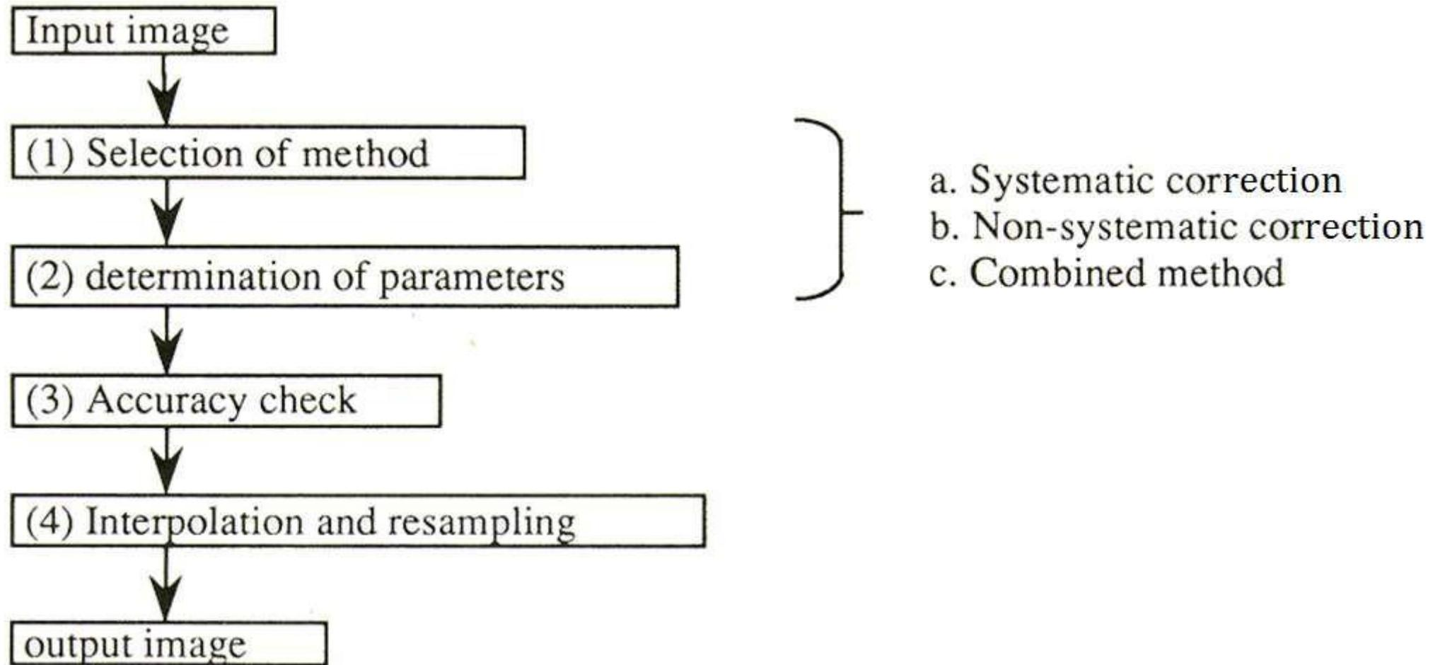
**Figure 1.9: The flow of geometric correction**
