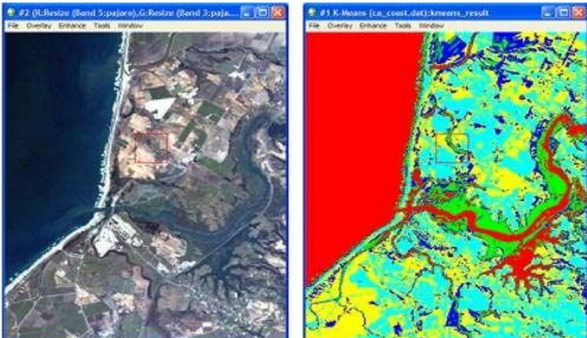
**Figure 1.22: In an unsupervised classification, a thematic map of the input image is created automatically in ENVI without requiring any pre-existing knowledge of the input image. The unsupervised classification method performs an automatic grouping; the next step in this workflow is for the user to assign names to each of the automatically generated regions (for example, the red class would be named “Water”)**
