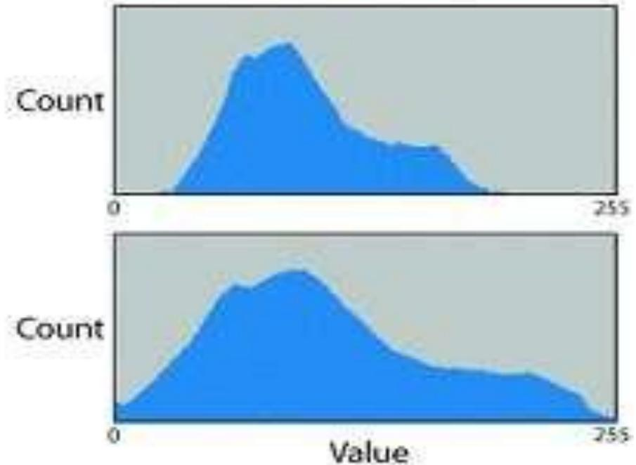
**Fig 1.10: It is an example of a contrast stretch. Histogram A represents the pixel values in image A. By stretching the values (shown in histogram B) across the entire range, you can alter and visually enhance the appearance of the image (image B).**
