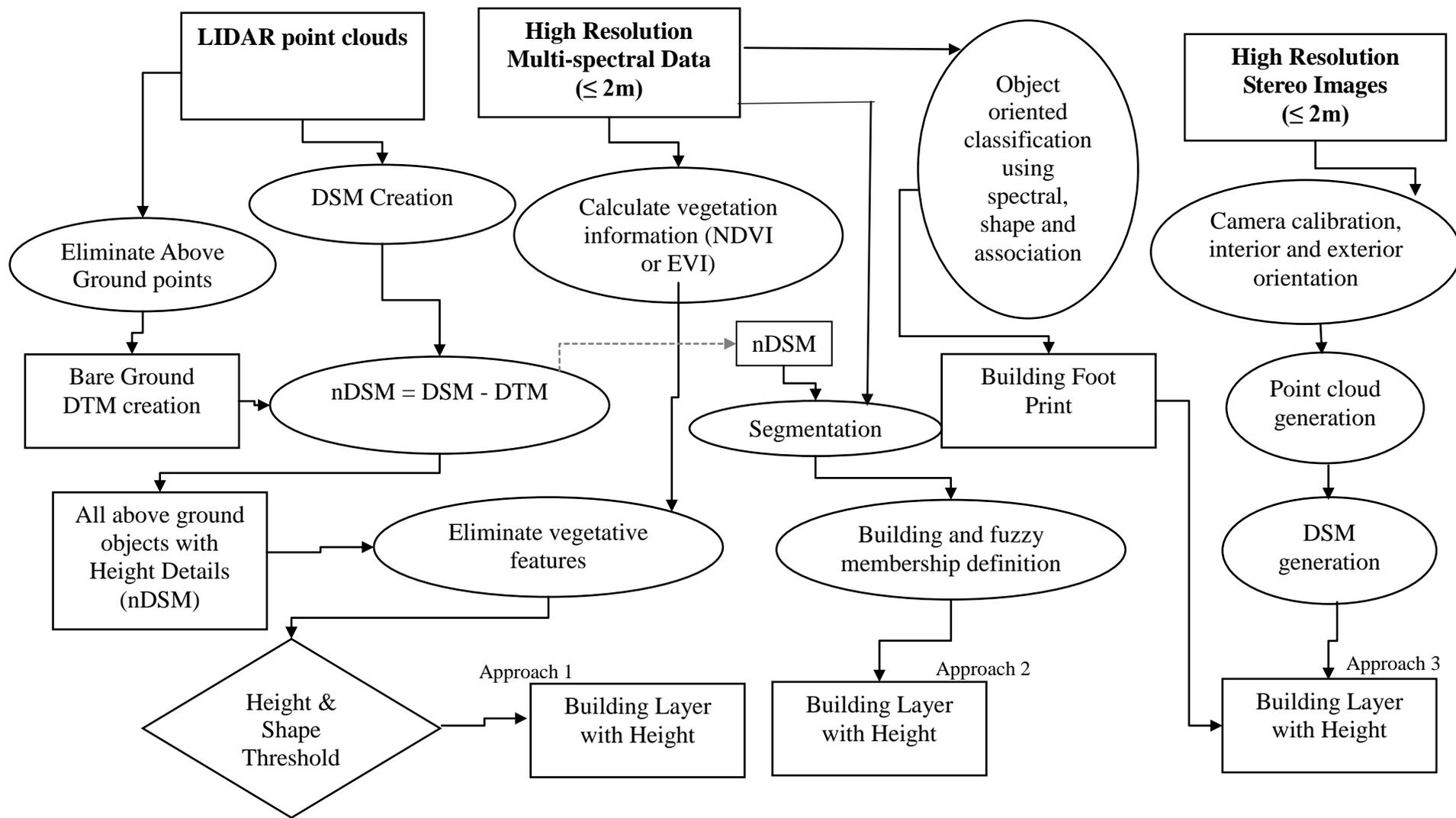
**Figure 4:** Building Extraction Process from Remote Sensing Data
