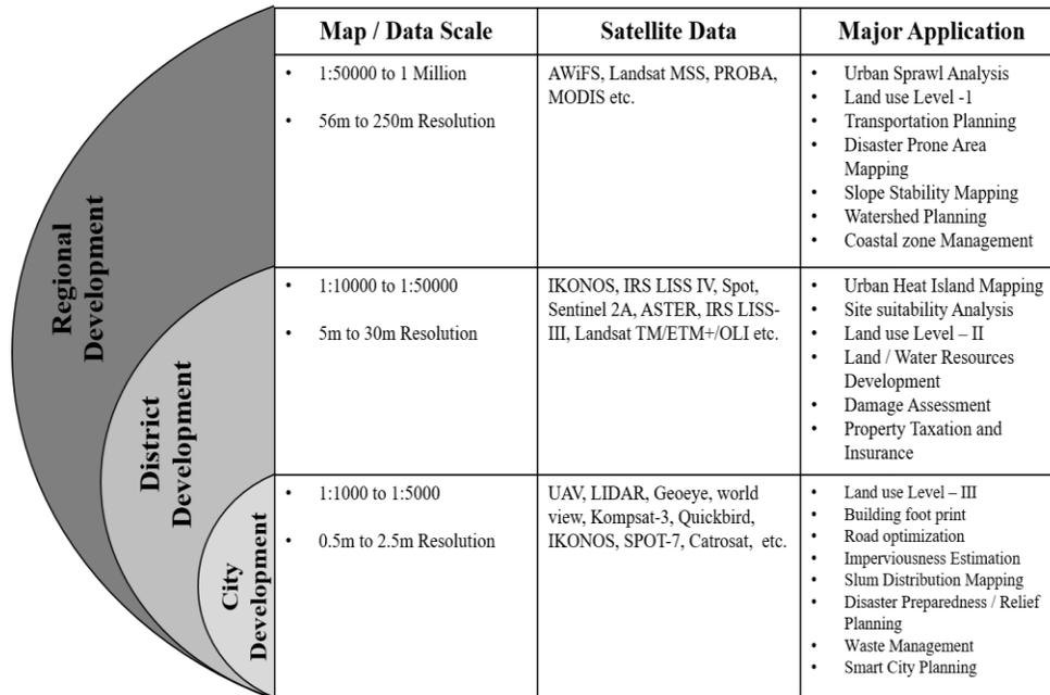
**Figure I:** Remote sensing based Civil Engineering Survey & Mapping Applications at Various Levels.
