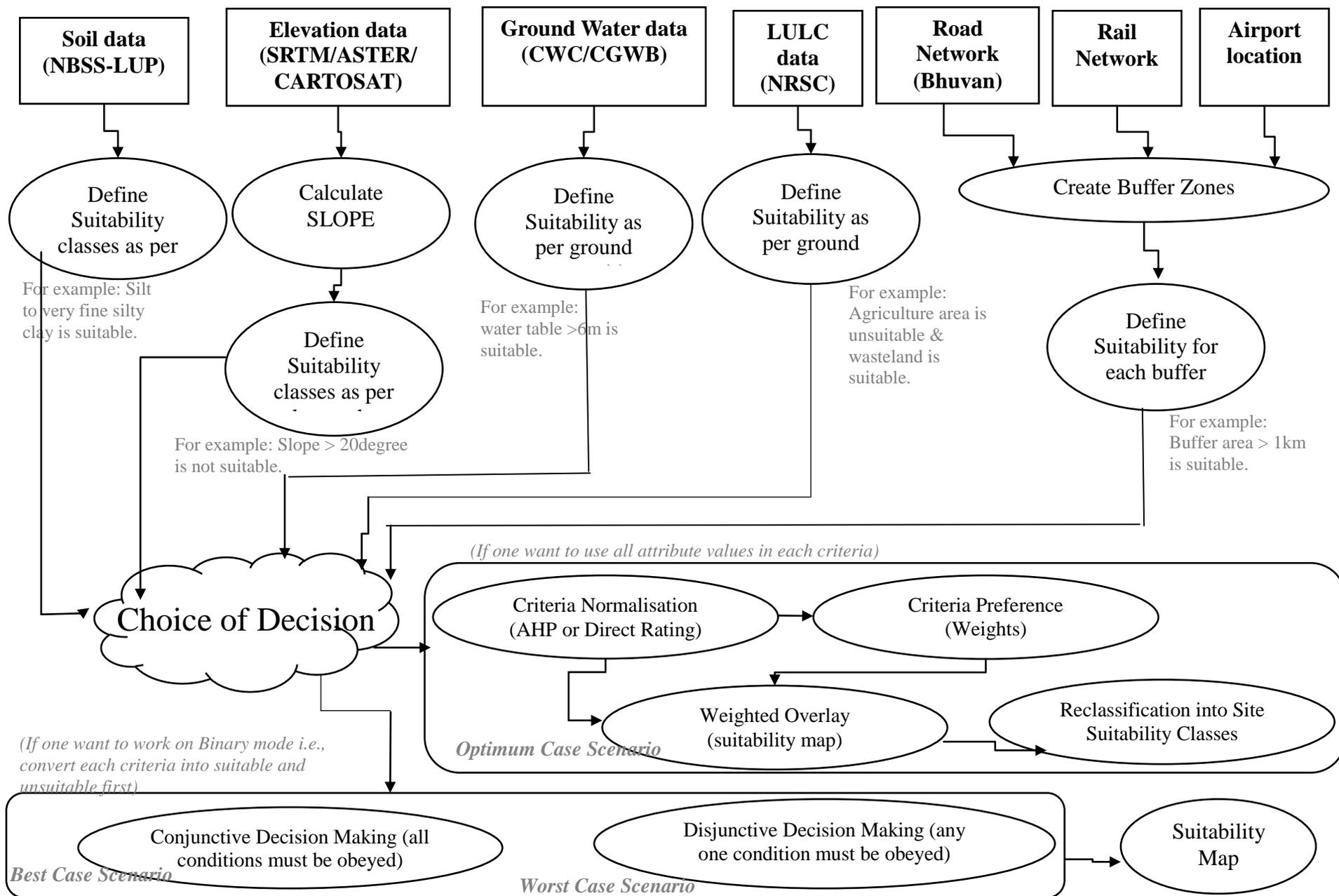
**Figure 6: Solid Waste Disposal Site Suitability Modelling using RS & GIS.** (NBSSSLUP – National Bureau of Soil Survey and Land Use Planning; CWC – Central Water Commission; CGWB – Central Ground Water Board; NRSC – National Remote Sensing Centre).
