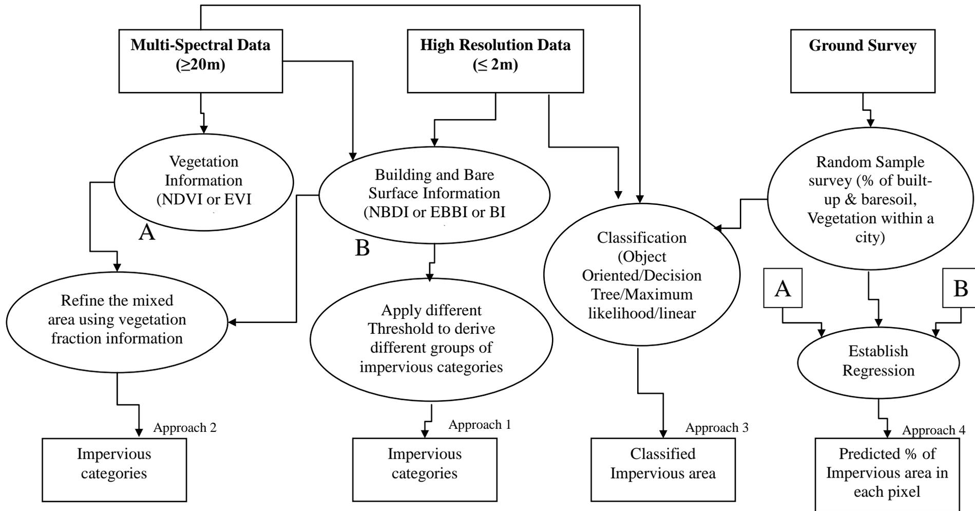
**Figure 2: Remote Sensing based approach for extracting Impervious Surfaces**
