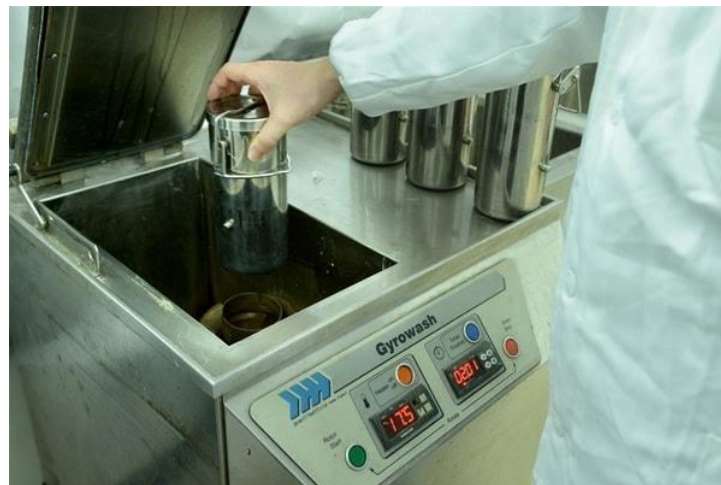
Fig: Washing fastness testing by Gyrowash
