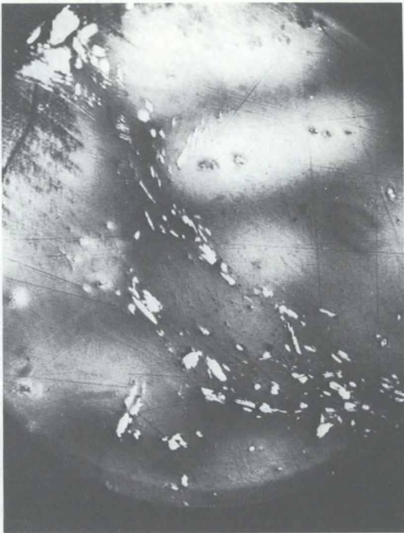
FIG.3. Photomicrograph (75x) of polished section of coalified uraniferous log collected in the Vanadium King No. 7 mine, North Adit, Middle Workings, Temple Mountain, San Rafael Swell, Emery Co., Utah. Log occurred in the Moss Back Member of the Chinle Formation (Triassic). Sample No. 7, 7.51% U, uraninite present. Coal preparation and photomicrograph by J.M. Schopf, US Geological Survey.
