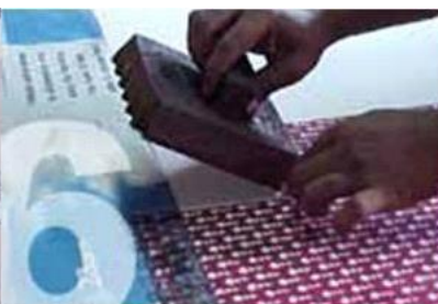
Fig 12: Step 6 – Printing of multi colour.
