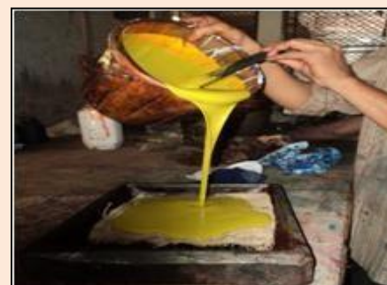
Fig 15: Step 2 – Transfer of the dye solution
