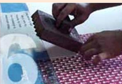
Fig 12: Step 6 – Printing of multi colour.
