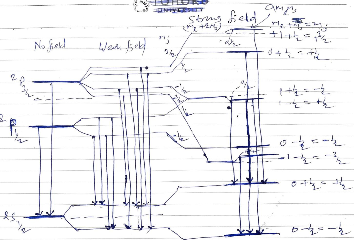
Energy levels for a principal series doublet starting with no field at the left and ending with a strong field (Paschen-Back effect) at the right.
