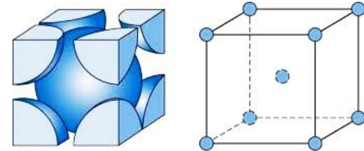
In the above figure, we can see that in a BCC structure,  $n=2$  because each of the corner atoms in a unit cell are shared by 8 other cells, whereas the one in the middle is not shared. Thus,  $n=(1/8) \times 8 + 1 = 2$
