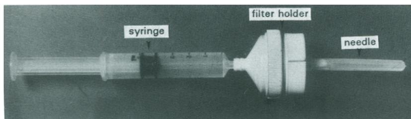
Fig. 2.3. 'Swinnex' Millipore filter assembly for sterilizing small volumes of liquids. The needle is not always required.
